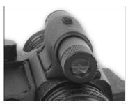
By pressing "SL" button three times you can switch to **Red diode** "I". **Red diode** represents 100M infra-red illuminator's brightness adjustment mode. Adjustments can be easily observed through the Aries scope while pressing" +" /" -" adjustment buttons.
